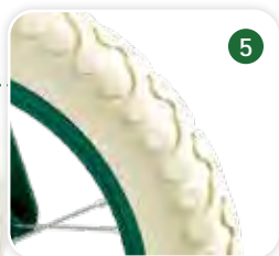
5 Lightweight, solid, puncture-free tires
